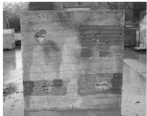
Fig.16 Surface treatment by water-jet (Rotary nozzle with 1 nozzle, 50 MPa, 19.2 l/min).
